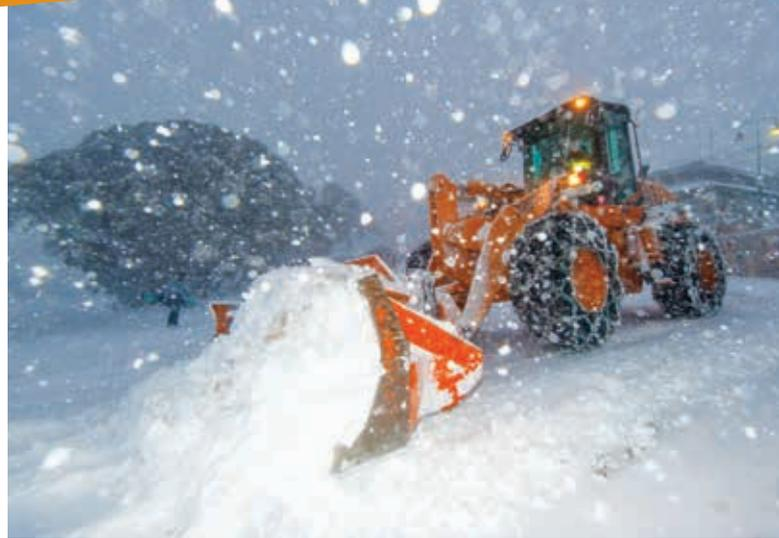
“When we get a huge dump of snow, we need to put chains on the Case 721F Wheel Loader’s tyres since the machines sometimes end up working on inclines that are basically made of ice,” noted Steve.
