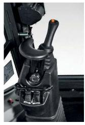
Rear pilot joystick as option. Standard: mechanical controls.
